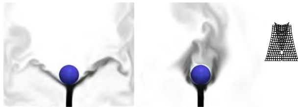
Fig. 10 We deform the grid to merge two branches of the smoke flow after it hits the sphere. Left: the original smoke animation without editing. Middle: the deformed smoke flow after editing. Right: the deformed grid, with discontinuous deformations.
