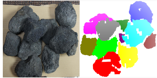
Fig. 9. Boularias et al. [12] performed instance segmentation (segments the pixels belonging to each object). For each instance, a set of push or grasp actions are sampled.
