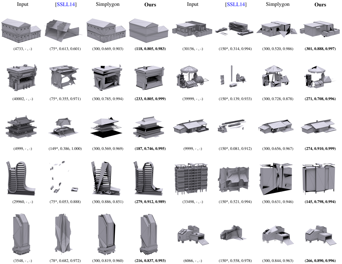
Figure 12: Our method compared with Simplygon and [SLL14]. (●, ●, ●) denotes (face number, recall, and precision).
