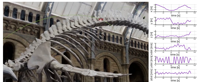
Fig. 4: Left: a simulation screenshot of the UAV (red) flies along a simulated trajectory that has neglectable differences from our optimized trajectory (green) in a museum. Right: each plot shows the overlaid positions ( x/y/z [m]) and the speeds ( \dot{x}/\dot{y}/\dot{z} [m/s]) of UAV for both the simulated and our trajectories.
